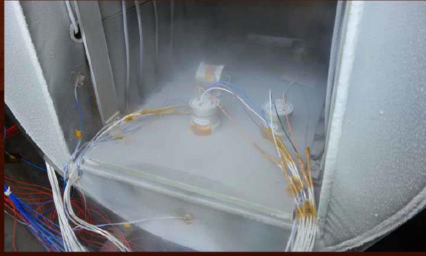
Rugged seismometers (qualified by JAXA to 2000-g for both the former Lunar-A mission and for terrestrial application) confirmed tolerance of Titan temperatures in tests at National Observatory of Japan in 2018. COTS geophones have similarly been tested in LN2 at APL and demonstrate excellent operation (minor damping change).
