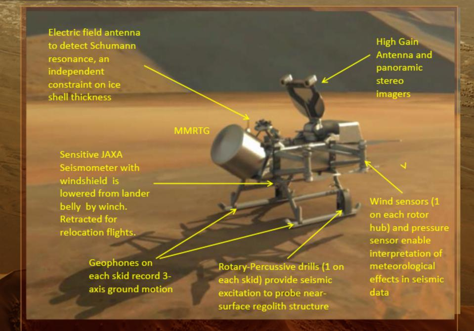
Geophysical and Meteorological instrumentation is integrated in a single package ("DraGMet") to facilitate synchronization and co-analysis of data from different sensors. Direct wind loads on deployable seismometer are eliminated by a wind shield, and lander noise can be decorrelated from seismometer signal by geophone records.
