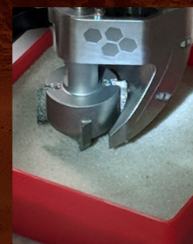
(Right) Cryogenic lab tests with Titan analog materials with a range of material properties show that the drilling system is capable of generating and transporting sufficient volume of tailings for sampling and analysis.
